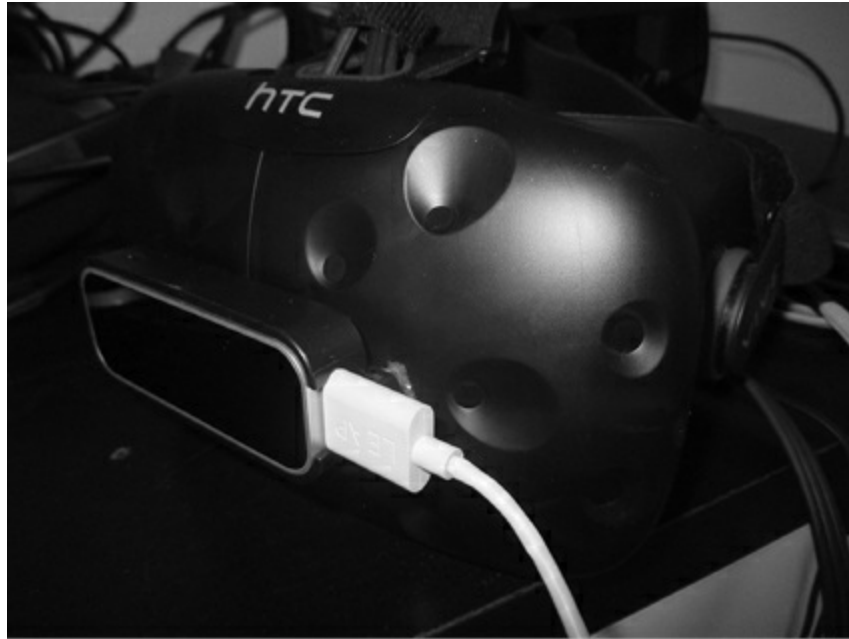
FIGURE 10.2 The VR mount kit provides a stable solution for attaching the Leap Motion device to a VR headset.
