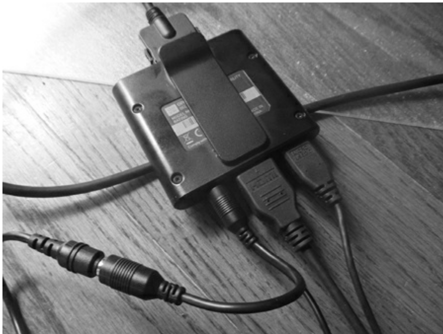
FIGURE 2.7 The beltbox for the HDK1.
